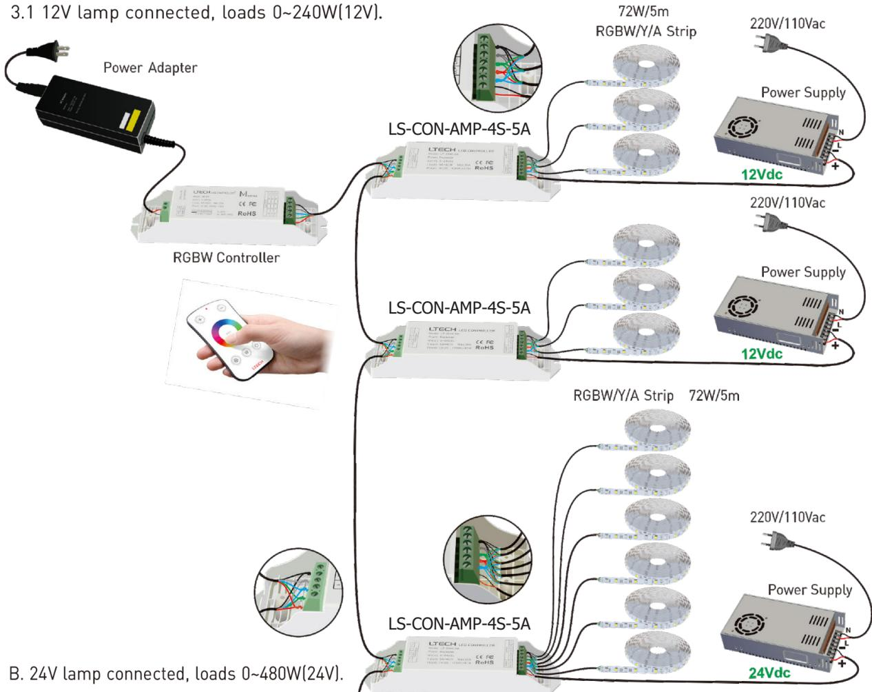
B. 24V lamp connected, loads 0~480W(24V).
