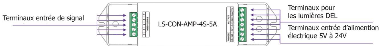
3.1 12V lamp connected, loads 0~240W(12V).
