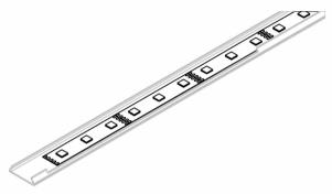
4. Once the strip is in place, press with your fingers along the whole length of the strip to ensure a good bond with the surface.
