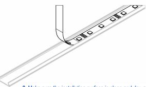
2. Make sure the installation surface is clean and dry, pull the protective film off et start applying the LED strip from one end.
